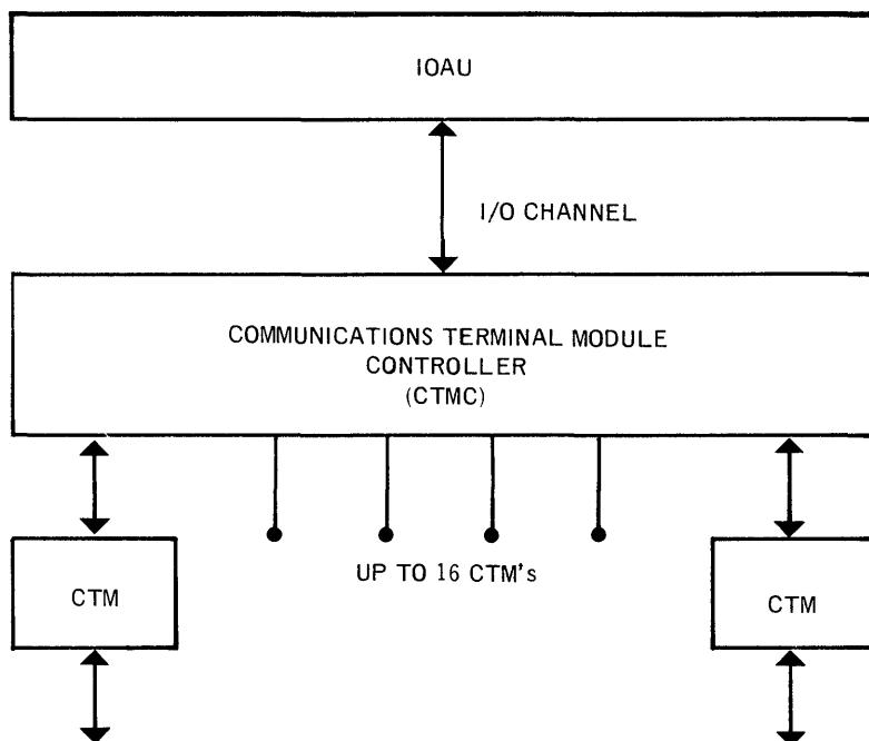
Figure 7-1. CTMC Subsystem, Block Diagram
