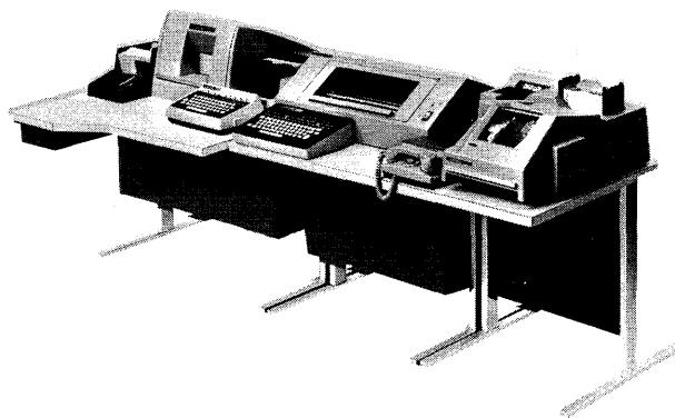
The Data Communication Terminal (DCT) 1000 is a fully buffered 30 character per second incremental printer which can be expanded to include a keyboard, card reader, card punch, paper tape reader/punch, and an auxiliary printer. The DCT 1000 transmits data or receives data from a local or remote computer or to a remote DCT 1000 in a conversational or batch mode.
