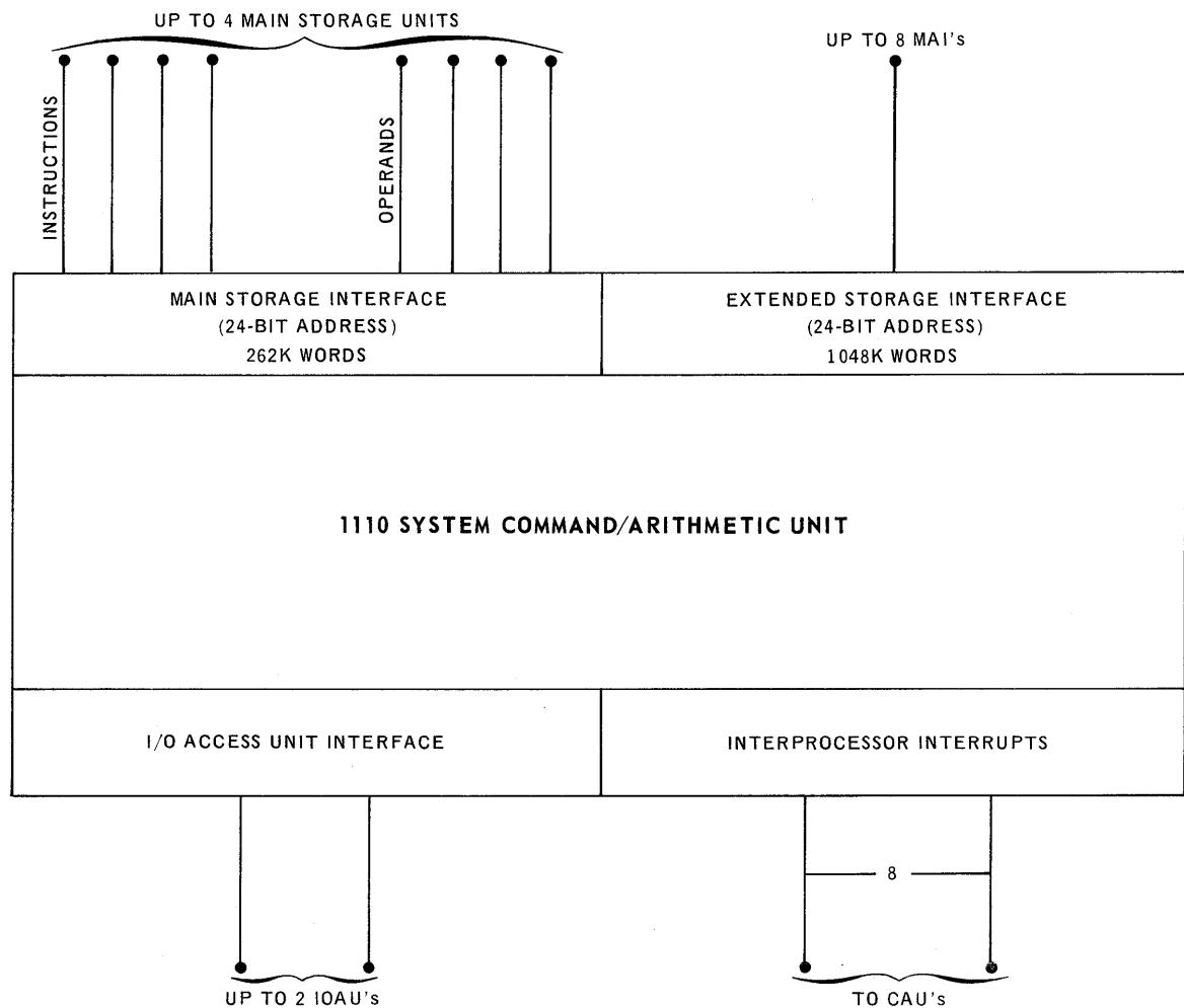
Figure 3-1. Command/Arithmetic Unit Configuration
