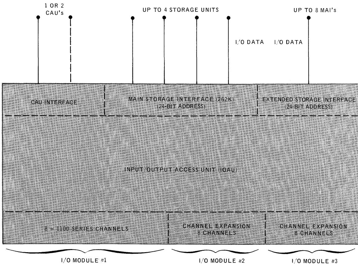
Figure 5-1. Input/Output Access Unit
