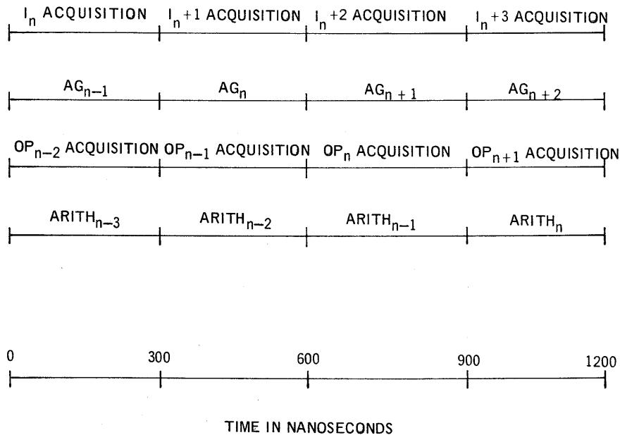
Figure 3-4. Instruction Execution (Approximate Timing) in a Command/Arithmetic Unit
