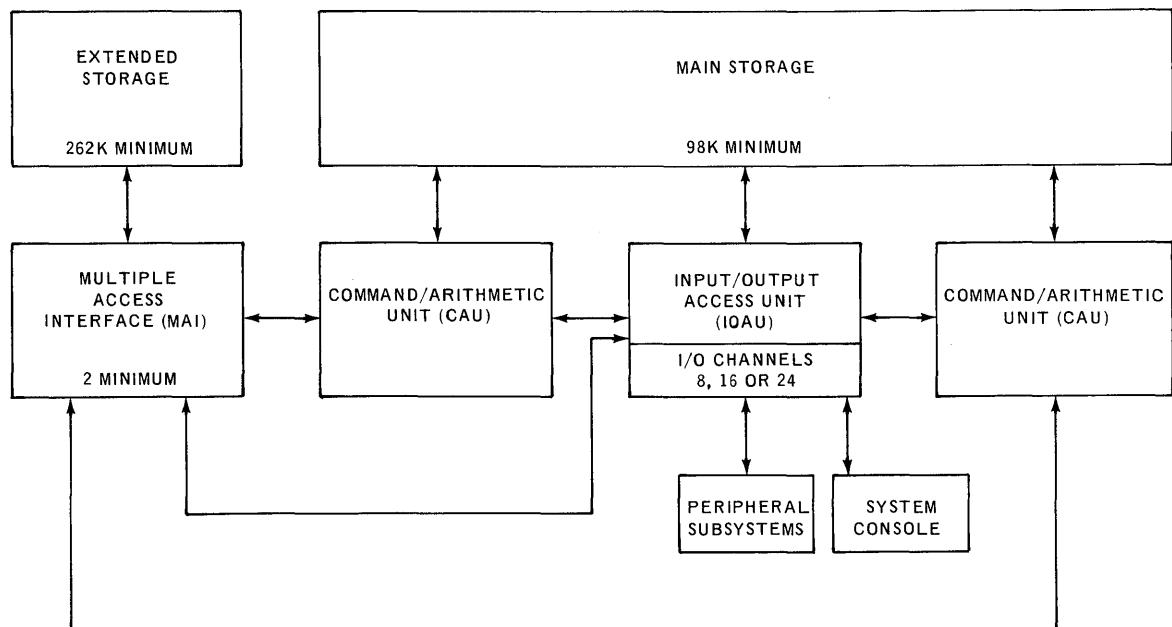
Figure 2-1. UNIVAC 1110 System, Basic Configuration (2 x 1)
