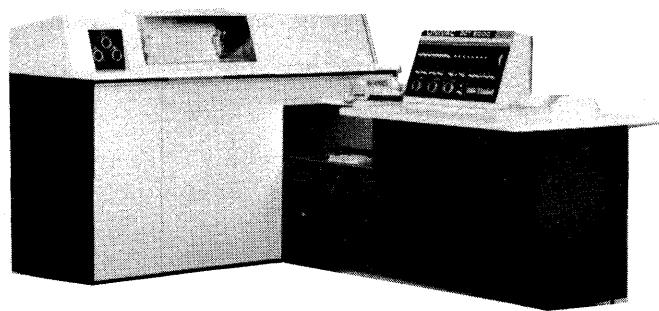
The UNIVAC Data Communication Terminal (DCT) 2000 is a combination printer and reader/punch designed to transfer large quantities of data efficiently over voice-grade facilities. This terminal (tied into a network with computers such as the UNIVAC 1004 Card Processor or other DCT 2000 systems) can handle up to 250 blocks per minute. The DCT 2000 is also available without the combination card reader/punch for use as a printer terminal.
