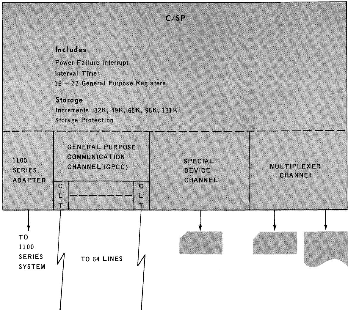
Figure 8–2. Communications/Symbiont Processor (C/SP) Configurator
